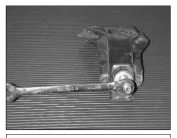
b. Using a 14mm wrench, remove the mounting stud from the factory engine mount assembly.
