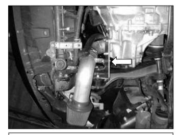
e. Install the lower intake pipe using the supplied coupler and hose clamps. Secure the intake bracket to the rubber mount using the supplied nylock nut and washer, as shown. Install the air filter and secure it with the supplied hose clamp.
