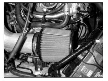
g. Install the AEM<sup>®</sup> filter on to the end of the inlet tube. Push the air filter over the inlet pipe until the "stop" in the air filter is reached. Install one hose clamp to secure the filter onto the inlet pipe. Once fitment is checked, you can either push the filter onto the inlet pipe more or less depending on clearances. Tighten the hose clamp after this is done.
