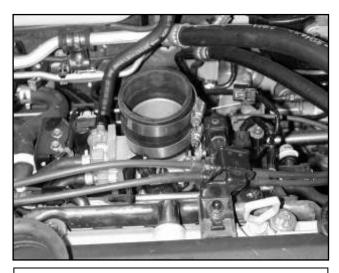
c. Install the  $2.5^{\circ}$  -  $2.75^{\circ}$  hose on to the throttle body using the  $2.5^{\circ}$  and  $2.75^{\circ}$  hose clamps. Check to see that the inside of the AEM<sup>®</sup> inlet pipe and air filter are clean and free from any foreign objects and/or obstructions.
