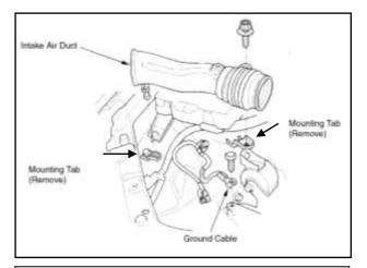
c. Remove the intake air duct by loosening the bolt at one end and then pulling the other end up out of the mounting tab. Remove the two intake air duct mounting tabs from the fender well.
