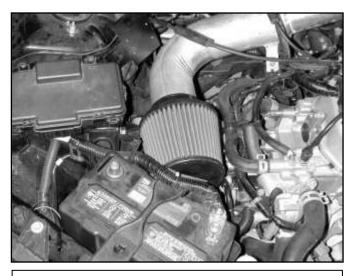
h. Ensure that the air filter is not touching any part of the vehicle. Position the inlet pipe for best fitment. Be sure that the pipe or any other component is not in contact with any part of the vehicle. Tighten the hose clamps at the throttle body and reducer coupling. Tighten the bolt on the intake resonator mounting bracket. Check for proper hood clearance. Re-adjust pipes if necessary.
