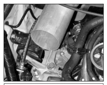
d. Slip the pipe under the cables and insert the small end of the pipe into the hose on the throttle body. The throttle body end is the end with the IAT sensor hole and breather hose nipple.
