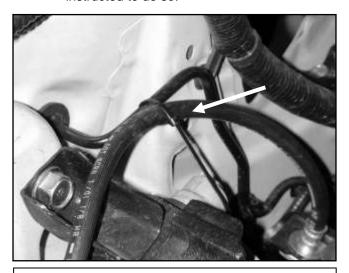
b. Use the supplied zip tie to secure the hydraulic hose, next to the shock tower, to the side and out of the way. Clip off the remainder of the zip tie when finished.
