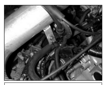
e. Thread supplied washer and bolt through the inlet pipe mounting tab into the factory intake resonator mounting bracket. Do not tighten.
