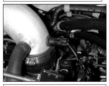
f. Install the supplied grommet into the IAT sensor hole in the AEM® intake pipe. Install the IAT sensor into the grommet and plug in the IAT sensor connector. Install the supplied 5/8" breather hose from the nipple on the intake pipe to the nipple on the valve cover. Use the supplied 1" hose clamp on the AEM® intake pipe nipple and the original hose clamp on the valve cover nipple.
