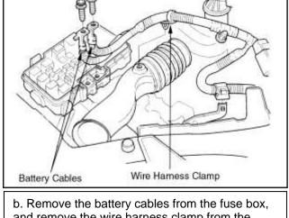
Remove the battery cables from the fuse box and remove the wire harness clamp from the intake air duct
