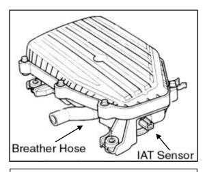
a. Make note of the location of the breather hose and intake air temperature (IAT) sensor.
