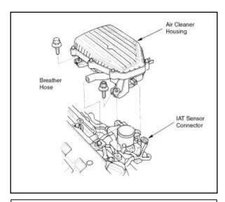
e. Remove the IAT sensor connector, than remove the breather hose. Loosen the hose clamp on the throttle body. Remove the air cleaner housing by removing the two bolts securing it. Remove the IAT sensor from the air cleaner housing (pull straight back) and set it aside in a safe place.
