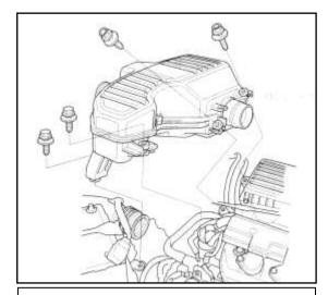
d. Remove the four bolts securing the intake resonator and pull the intake resonator out of the car.
