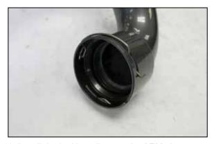
14. Install the locking clip onto the AEM charge tube as shown.
