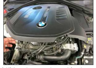
2. Lift the engine cover and remove it from the vehicle.
