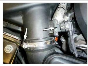
3. Disconnect the mass air sensor electrical connection and loosen the hose clamp that secures the intake hose to the air filter housing.
