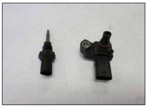
11. Remove the temperature sensor and pressure sensor from the factory charge tube.
