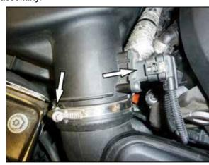
23. Reconnect the mass air sensor electrical connection and connect the intake tube to the air filter housing and secure with the factory hose
