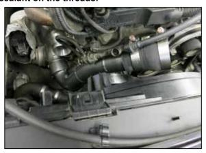
17. Install the step hose onto the lower charge tube section but do not tighten the clamp at this time. Install the lower tube section onto the turbo outlet, push the pipe on until the locking ring "clicks" into the locking groove.
