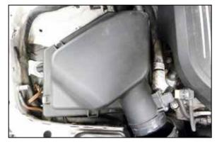
4. Lift the air filter housing up to dislodge it from the mounting grommets and remove it from the vehicle.
