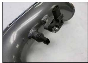
15. Install the temperature sensor and pressure sensor into the AEM charge tube.
