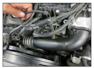
6. Disconnect the charge tube pressure and temperature sensor electrical connections.
