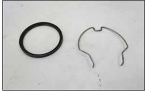
12. Remove the O-ring and locking clip from the factory charge pipe.
