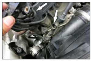
9. Disconnect the vacuum switch from the ccv line as show to allow clearance for the charge pipe to be removed.
