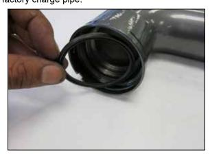
13. Install the factory O-ring into the AEM charge tube.
