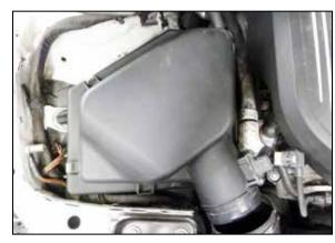
22. If not installing a AEM intake system, Reinstall the factory intake tube and air filter housing assembly.
