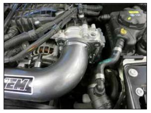
18. Install the upper AEM charge pipe into the coupler and then align with the throttle body, Secure the pipe to the throttle body with the factory bolts.
