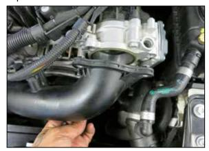
7. Using a T30 torx bit remove the three bolts that secure the charge tube to the throttle body.
