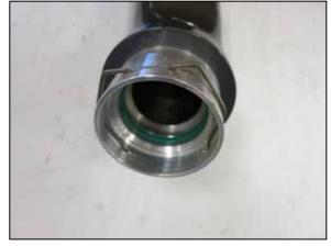
14. Install the factory O-ring and retaining clip into the AEM charge pipe as shown.
