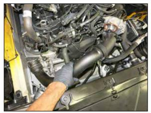
6. Separate the charge pipe from the turbo charger and then remove it from the vehicle.
