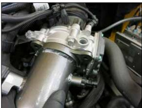
15. Install the AEM charge pipe onto the turbo inlet and throttle body. Push the tube onto the turbo until the retaining ring locks it into position while also aligning the top of the pipe with the throttle body.
