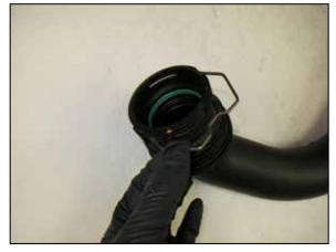
7. Remove the retaining clip from the stock charge pipe and set aside to be used with the AEM charge pipe in a later step.
