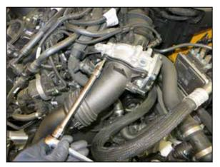
4. Remove the three bolts that secure the factory charge tube to the throttle body.
