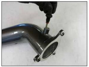
13. Install the inlet air temperature sensor into the AEM charge pipe.
