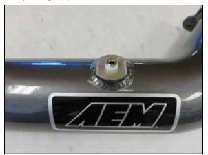
11. Install the 1/8npt pipe plug into the accessory port of the AEM charge pipe. Be sure to apply thread sealer to the plug before installation. Install the AEM decal as shown.
