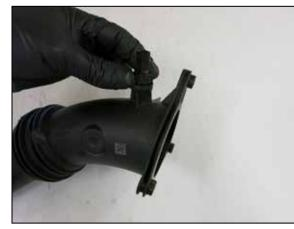
10. Remove the inlet temperature sensor from the factory charge pipe.
