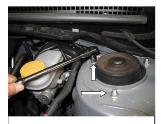
a. Remove the 2 Strut Tower nuts from each side needed to install the AEM Strut Tower bar.
