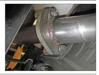
g. Ensure the bolt/nut assemblies are tightened to factory torque specification (see service manual).
