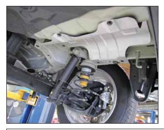
e. Remove the OE muffler, ensure the exhaust gasket is removed and set aside. The gasket will be reused during the installation of the AEM<sup>®</sup> exhaust system.
