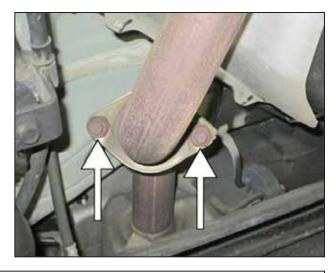
b. Remove the two nuts securing the muffler pipe to the exhaust pipe.
