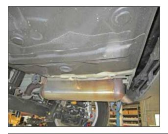
a. Stock exhaust system installed.
