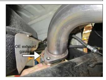
e. Install the OE exhaust gasket between the OE exhaust pipe and the AEM<sup>®</sup> exhaust pipe.
