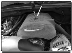
**25.** Install the provided 8mm hose to the fitting on engine, and connect to the fitting on the intake tube.
