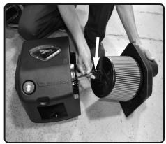
**3.** Connect the 3 mm Vacuum line to the 5/32" fitting on the top of the filter.
