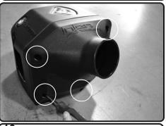
**18.** Now secure the plenum using provided 4 M6 screws and rubberized washers. Secure and tighten.
