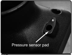
17. IF vehicle is equipped with pressure sensor, drill hole out 1/4" and install to plenum. Do not drill if vehicle does not have temperature sensor.
