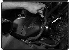
**23.** Install the 4" hump hose to the plenum. Tighten clamp on plenum only.
