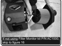
**15.** Attach the other end of the 3mm vacuum line to the filter fitting and secure.
