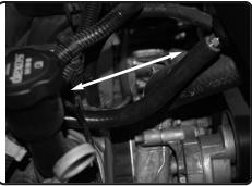
**26.** Install the provided 8mm hose to the fitting on engine, and connect to the fitting on the intake tube.
