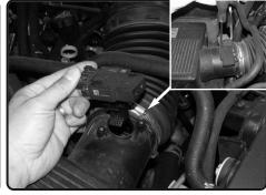
**4.** ∪s a T15 Torx bit and remove the two screws on the MAF sensor. Pull the MAF sensor out of the factory air box assembly
