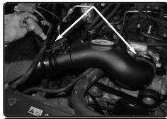
**24.** Install the intake tube. Position for best fit, secure and tighten all clamps using 8mm nut driver.
