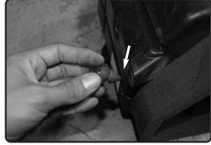
**10.** Remove the grommet spacer from the factory air box.
