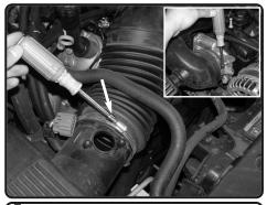
**5.** Use a 8mm nut driver and loosen the clamp on the intake air duct from the air box assembly and clamp on throttle body.
