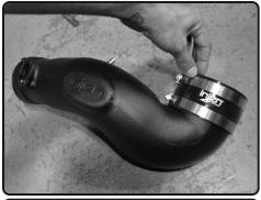
**19.** Install the the 4" straight hose to the tube with clamps provided.
