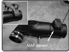
**20.** Install the MAF sensor into the intake tube and secure using provided M4 button head screws.
