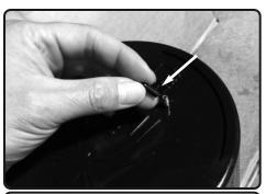
**13.** Place the 3mm vacuum cap on top of the Injen filter if you are not using the optional Filter Monitor Kit P/N AC1000
