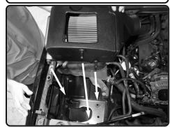
**21.** Now install the air box assembly into the vehicle. Position the tabs to seat like OEM box.
