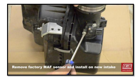
14. Reinstall your MAF sensor into the new GrimmSpeed tube using the included machine screws and your 3mm allen wrench. The MAF can only be installed in one direction, so there's no need to worry about accidentally installing it backwards.
