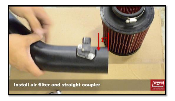
16. Finally, use your 5/16" socket to tighten the filter onto the intake tube, ensuring that it is straight.
