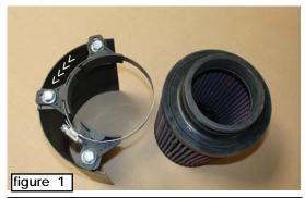
The HS-brackets are set over the press nuts and fastened with the 5/16" bolts.
