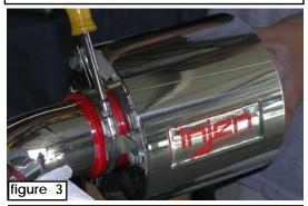
Once the filter is aligned continue to tighten the clamp over the intake.
