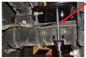
check driver's and passenger's sides to make sure the hard brake line is not rubbing on the carriage bolts. Adjust by pushing on the line to gain clearance if necessary.
