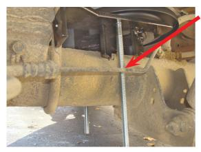
Carriage bolt must be between the hard brake line and axle for this model that has the brake line routed off the axle.
