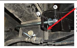
Draw hardware evenly (snug only, do not tighten yet) making sure the lower bracket stays in position and locked around the U-bolts.
