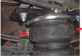
Once tight, the upper and lower brackets will not be parallel and may look like they are out of alignment. This condition is acceptable because of the way the lower bracket and upper bracket mounts are designed. Some variance from one unit to another is considered normal (Fig. C.20).
