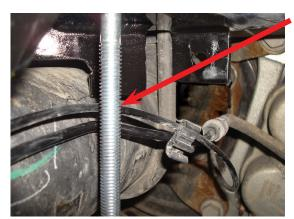
The carriage bolt is always on the outside of the brake line on the passenger's side, regardless of the year.
