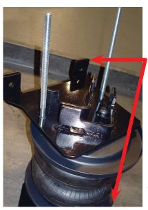
The flanges on the lower bracket must be on the opposite side of the fitting that is on the top of the air spring assemblies.
