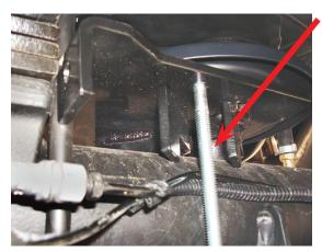
Carriage bolt must be on the outside of the hard brake line and axle for this model that has the brake line flush to the axle.
