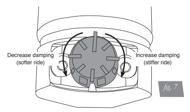
2. Next, completely deflate and reinflate the air bags 2-3 times. This procedure will purge any trapped air in the dampers and allow for maximum performance. For ride performance and the most versatility, Lifestyle recommends setting the strut dial (if equipped) to position 6 or higher.
