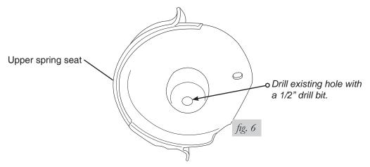
8. You will need to drill a hole through the upper spring seat frame reinforcement in order to gain access to the cylinder for the hose. Measure up from the bottom edge of the reinforcement 3.5" at the center of the spring (fig. 7).
