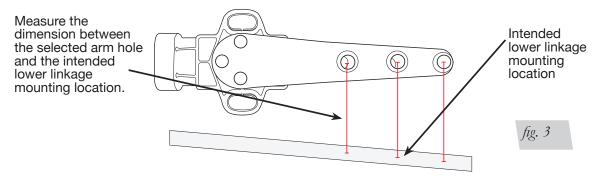
Reinstall air lines and cycle the suspension to get to the upper limit position again, measuring between the sensor arm's middle position and directly below the sensor arm hole mounting to the lower linkage ball joint (fig. 4). The difference between these two values will be the full suspension travel range.
