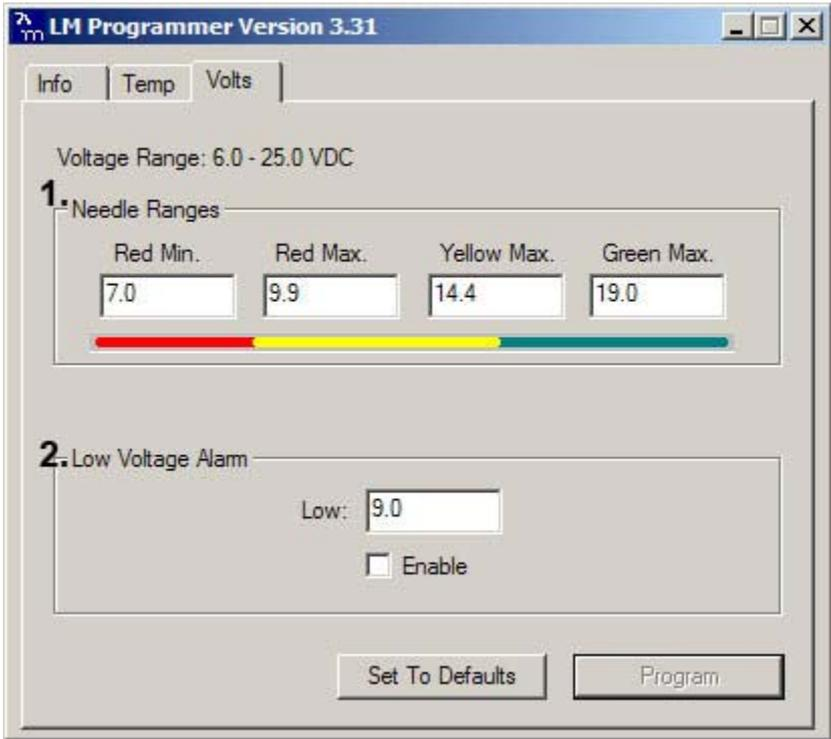
1. The **Needle Ranges** allows the configuration of each outer LED segment. The voltage range displayed is user defined.
