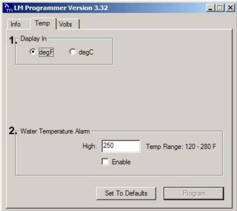
1. The **Display In** will allow the gauge to display the temperature in either Imperial or Metric unit of measure.
