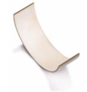
A lead free silver based overlay material containing solid lubricant additives distributed throughout the silver matrix. For extreme load engines. Can be used as a sputter replacement.
