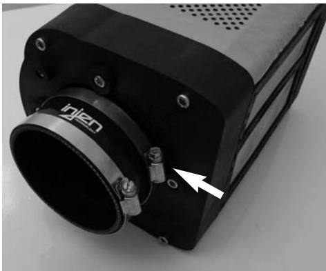
The four inch hose is pressed over the velocity stack outlet. Use two large clamps, one on each end of the hose and tighten the clamp on the velocity stack outlet.
