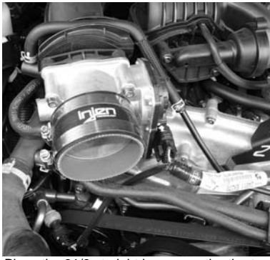
Place the 3/8 straight hose over the throttlebody and place twomedium (362) clamps over the hose, tighten only the clamp on the throttlebody side for now
