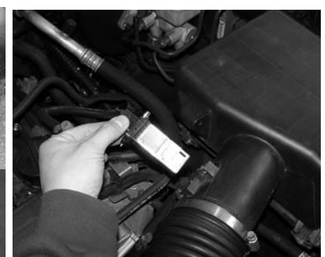
Now remove the MAF sensor out of the factory air box sensor housing. This MAF sensor will be reused later.
