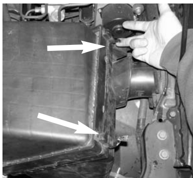
Unclip two retaining tabs holding the upper part of the air box to the lower part of the air box
