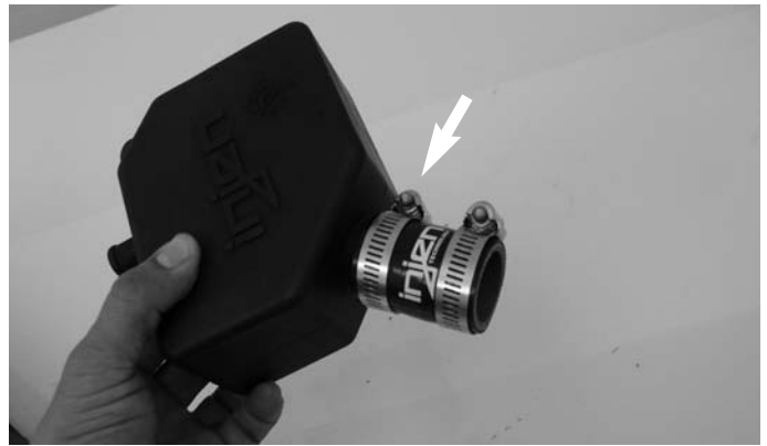
Once both clamps have been placed over the hose be sure to tighten the first clamp nearest to the CCV box.
