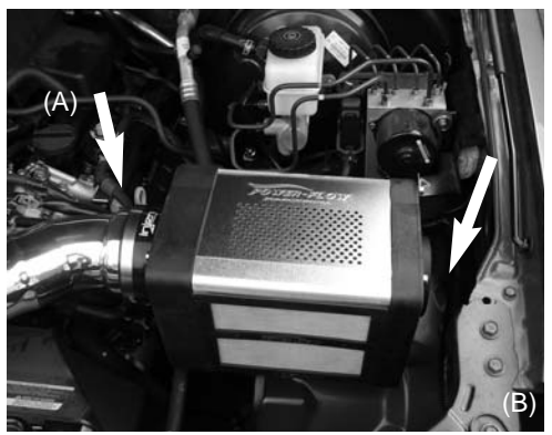
The four inch velocity stack base is connected to the intake (A) and the Power box bracket is lined up to the vibra-mount stud (B).
