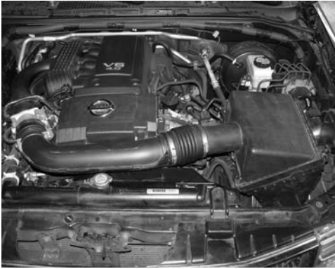
Picture of factory air intake system
