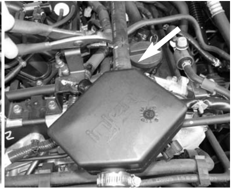
Insert crank case breather line over CCV box port and use stock clamp to secure breather line.
