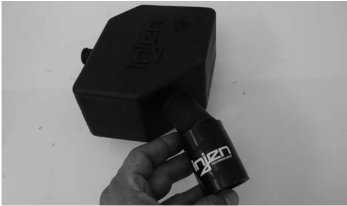
Take the CCV connecting hose and press it over the CCV box large port. Two clamps will be placed over the hose.
