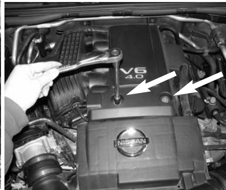
Use a 10mm socket with a 3/8 ratchet and remove the two 10mm bolts on the engine cover.
