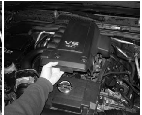
Lift up and pull towards you to remove the engine cover. This cover is removed to access the two 10mm bolts to the air duct resonator box/
