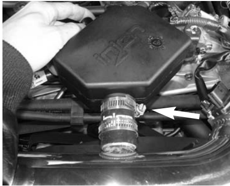
Press the CCV box over the large intake port, adjust and tighten clamp as shown in the picture.
