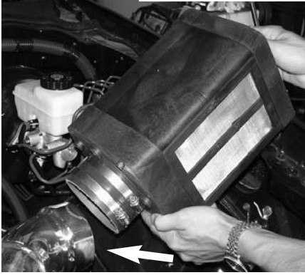
Position Power-flow box in the engine compartment and press four inch hose over the intake inlet as shown in this picture .
