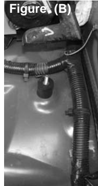
Place the vibramount onto the pre-tapped hole located next to the ABS solenoid pump. (Figure A) Vibramount mounted on pre-tapped hole. (Figure B) This vibramount will be used for the mount point for the Injen airbox.
