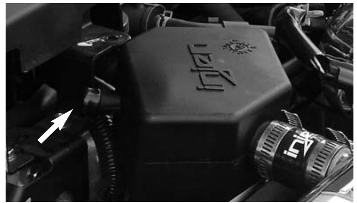
Side shot of CCV box vacuum cap and CCV box installed.
