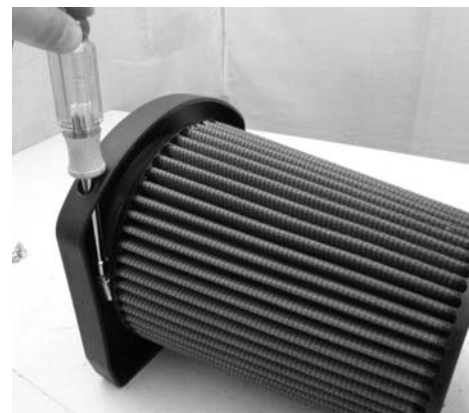
Loosen the clamp on the filter neck in order to separate the filter from the velocity stack.
