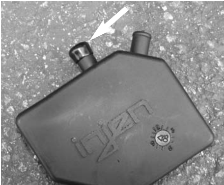
Press CCV box 5/8" vacuum cap over left port which will not be used.
