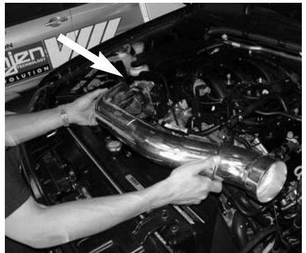
Lower the Injen intake pipe into the engine bay and place the 2.75" pipe end into the 2.75" straight hose already on the throttlebody.
