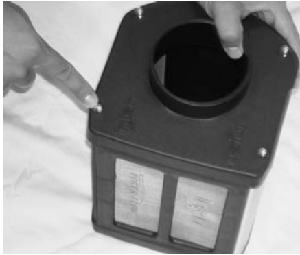
Here are the four-m6 x 20mm bolts that will be removed from the velocity stack base located on the corners of the base.
