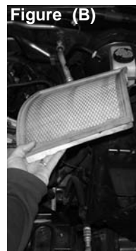
Remove upper part of air box (Figure A) and remove panel filter to get to 10mm bolt located inside of air box (Figure B)
