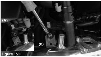
Line up the solenoid with the locating pre-drilled tab to the bracket located on the intake. Use the m6 x m16 bolt and flange nut to fasten the solenoid to the bracket (B). Some models may not have this solenoid. If your vehicle is not equipped with this solenoid, please skip to figure 6
