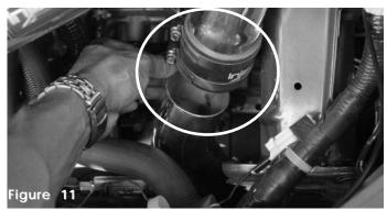
The secondary intake will come up into the engine compartment. Line up and insert the top section of the secondary intake into the end of the primary intake. Press the primary and secondary intake together and semi-tighten the clamp.
