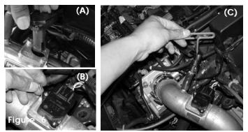
Insert the mass air flow sensor into the machined adapter on the intake and locate in place (A). Use the two supplied M4 bolts to fasten the sensor into the machined adapter (B). Use a 2.5mm allen driver to tighen the M4 bolts to the MAF (C)
