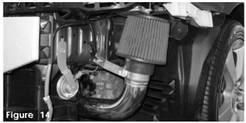
Press the filter neck over the end of the secondary intake and tighten the clamp on the filter neck.
