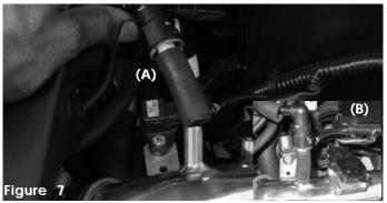
Take the 2 inch-10mm coupler and press it over the air temperature sensor (A). Press the coupler with the air temperature sensor over the 1/2" port on the intake (B).
