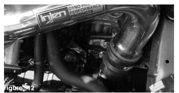
View of the primary and secondary intake butted up together.
