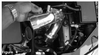
Insert the primary intake into the engine compartment and insert the top end into the 2 3/4" hose on the throttle body. Semi-tighten the clamp on the intake side just to hold it place.
