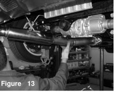
Position the rear section of the Injen exhuast system
