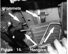
Attach the hangers onto the grommet on the rear section of the Injen exhaust system
