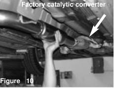
Position the primary Injen exhaust pipe and attach the flanges end to the factory catalytic converter
