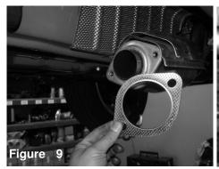
Place the supplied 3.00" gasket onto the catalytic converter
