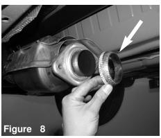
Remove the donut gasket from the factory catalytic converter
