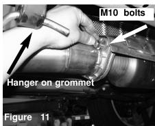
Place two M10 bolts to attach the Injen primary pipe to the factory catalytic converter. Remember to place the two hangers on the Injen primary pipe
