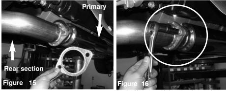
Once the rear section is hung and in position, place a 3.00" gasket inbetween the primary and rear section
