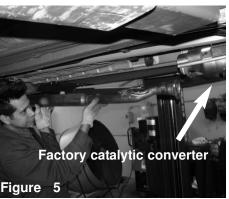
Detach the primary exhaust section off of the catalytic converter
