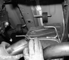
Pull all exhaust hangers off of factory exhaust system
