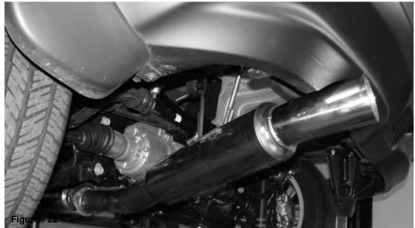
Congratulations! You have just completed the installation of the Injen cat-back exhaust system. Periodically, check the fitment of the exhaust system, the exhaust should always continue to hang in the same position.
