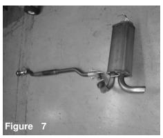
Factory exhaust system fully detached in one piece
