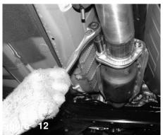
Use a 14mm socket and rachet and tighten the M10 nuts and bolts
