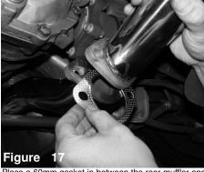
Place a 60mm gasket in between the rear muffler and mid-pipe on both left an right side.
