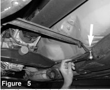
Use a 10mm socket and rachet to remove the two 10mm bolts attaching the brace bar to the right/left skid plates. Drivers side shown
