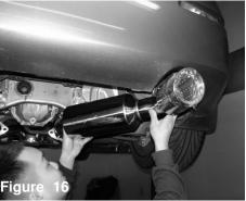
Place the rear right and left mufflers onto the hangers
