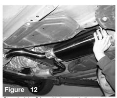
Place the Injen Primary X-pipe onto the factory catalytic converters. Re-use the four factory M10 nuts to secure Injen X-pipe to the cats
