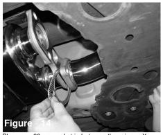
Place one 60mm gasket in between the primary X-pipe and right side mid-pipe and repeat for the left side.
