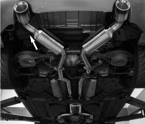
Congratulations! You have just completed the installation of the Injen cat-back exhaust system. Periodically, check the fitment of the exhaust system, the exhaust should always continue to hang in the same position.
