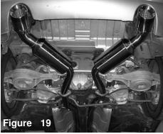
The rear mufflers are now installed. Make your final adjustments for best fitment and then tighten all M10 bolts
