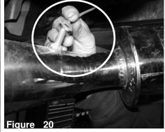
Connect the grounding wire located at the rear of the vehicle to the welded bolt on the driverside muffler piping.
