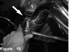
Now position the exhaust for best fit and clearance. Secure and tighten using 17mm socket and ratchet.
