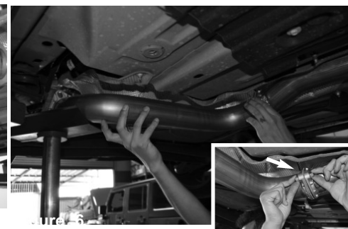
Figure 6 Once the mid-pipe is in place. Use provided 76mm gasket and 2 bolts and nuts. Do not tighten.
