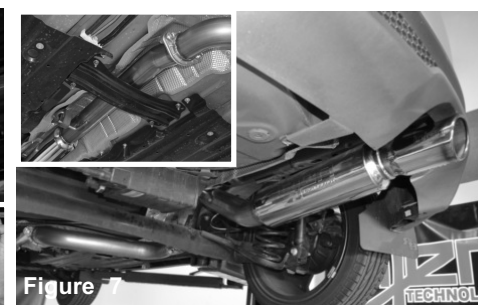
Figure 7 Install the rear section and position to mid-pipe. Use provided 76mm gasket and 2 bolts and nuts. Place the metal hangars into the rubber isolators. Now position and tighten using 14mm socket and wrench. Tighten nuts on flange from step 4. Re-install the bracket from step 2, make sure there is clearance. Re-adjust if necessary. Note: Flanges have room for rotation, if exhaust comes close to touching any other component, adjust and move flanges to get proper fitment.
