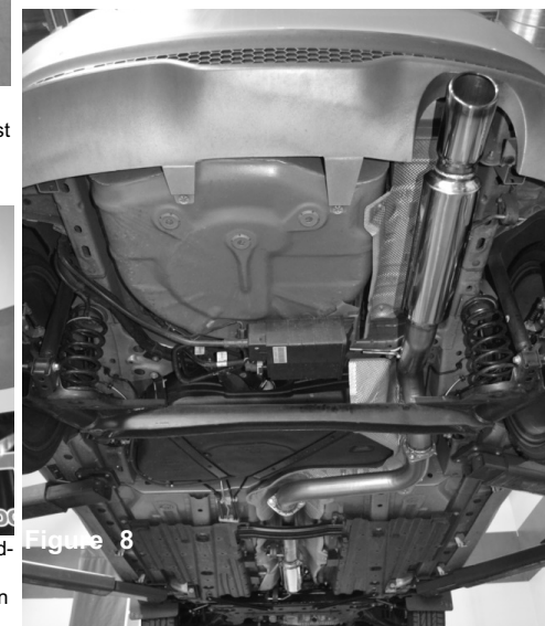
Figure 8 Make sure nothing comes into contact with any component and then make your final adjustments to the entire exhaust system. Use a 14mm socket and ratchet secure all the M10 nuts and bolts. Congratulations! You have just completed the installation of the Injen Cat-back system. Periodically, check the alignment of the exhaust, normal heat cycles can cause nuts and bolts to come loose. Failure to check the alignment and adjust the exhaust can cause damage that will void the warranty.
