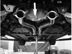
Now install the mid-pipes to the Y-pipe. Install the hangars to the rubber isolation mounts. Secure using provided 3" gaskets and bolts with nuts. **Do not tighten.**
