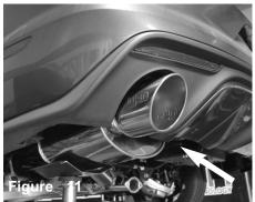
Install the rear section. Install the hangars to the rubber isolation mounts.
