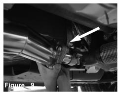
With gasket, install the Y-pipe to the adaptor. Secure using provided M10 hardware. *Do not Tighten.*
