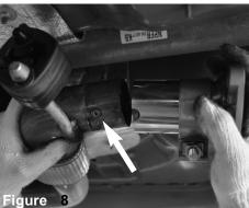
With exhaust removed, now install the adaptor with provided band clamp to the OEM downpipe. Make sure the slot cut out matches to the fitting on the stock down pipe and locks. Tighten band clamp using 17mm socket or wrench.
