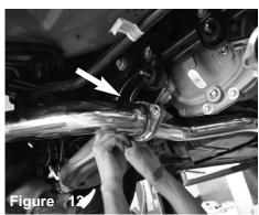
Secure using provided 3" gaskets and bolts with nuts. *Do not tighten.*
