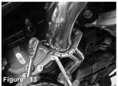
Snug fit all bolts and nuts using 14mm socket or wrench. Adjust for clerance and fitment. Make sure tips are centered of exhaust hole cut-out on bumper. Re-adjust if necessary. Use and extra hand for position of muffler and tighten all bolts and nuts.
