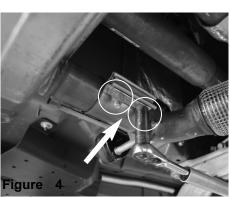
Loosen the 2 15mm nuts on the band clamp on OEM down pipe. Loosen and pull back.
