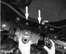
Remove the hangers from the factory exhaust. Use lubrication for easier removal. Re-install the rubber isolation mounts to vehicle and secure.
