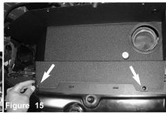
Figure A: The lower intake pipe should be perfectly in the Place the two .242" Click lock Rivet into the two .250 center of the 4" hole on the lower air box. Figure B: If the holes in front of the lower air box.
