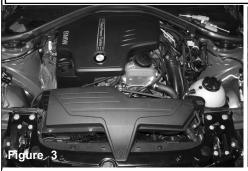
Stock air box assembly shown in this picture. Disconnect pattery before the install.
