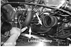
Use a 7mm nut driver to loosen the clamp on the lower turbo air duct. The upper air duct will be removed from the engine bay and no longer be used.
