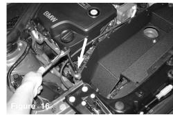
Place a M6 nut and fender washer onto the stand off and secure the nut to the lower air box bracket. Your lower air box is now secured to the vehicle.
