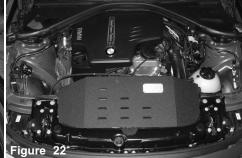
Push the front OE mounting grommet down onto the front Congratulations! You have just completed the installation OE air box mounting stud. Place the air box cover on top of this intake system. Periodically, check the alignment of of the lower air box and place four supplied M6 allen bolts the intake, normal wear and tear can cause nuts and bolts to come loose. Failure to check the alignment and adjust the intake can cause damage that will void the warranty.
