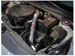
24.Ensure that all bolts, clamps and hoses are properly secured.
