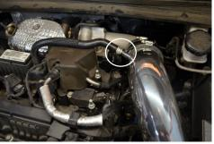
17. Reattach the crank case hose to the injen tube, then secure the hose with the OEM tension clamp.
