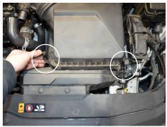
6. Disengage the two clips securing the upper airbox housing.
