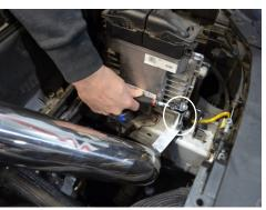
14. Next, attach the tube to the step hose. 15. Line up the bracket to the vibra mount, then secure the bracket with the provided M6 nut and washer.
