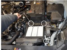
8. Remove the two push clips securing the 9. Remove the three bolts securing the airbox.
