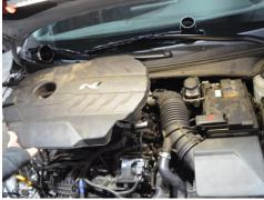
2. Remove the engine cover by firmly lifting it on all four sides.
