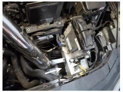
13. To install the Injen intake tube. First, route the tube below the chassis rail.
