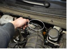
5. Loosen the clamp securing the OEM tube to the turbo inlet, then detach the tube.
