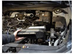
10. Remove the bottom airbox assembly.
