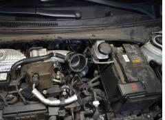
11. Place the provided step hose on to the turbo inlet. Only secure the clamp on the turbo inlet for now.
