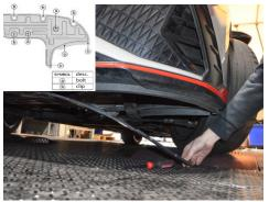
20. Remove the bolts and clips indicated on the diagram in order to detach the under cover enough for the air filter.
