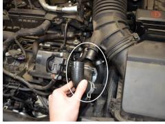
4. Disconnect the diverter valve hose.
