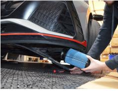
21. Pull down the under cover, then insert 22. Secure the air filter to the intake tube the air filter through the bottom front bumper.
