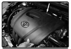
**25.** Re-install engine cover. Re-connect battery ..
