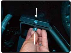
**19.** Secure using provided M6 screw and nut.
