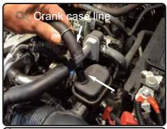
**3.** Push the factory clamp in and pull back the crank case line away form the intake tube.
