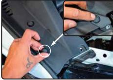
**12.** Push down on the clips on the radiator cover, remove clips and guard for installation of heatshield.
