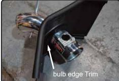
**10.** Install the intake tube through the hole with MAF sensor pad side. Maneuver and finish the rest of the bulb edge trim installation.
