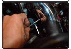
**21.** Re-connect the OEM vacuum line to the fitting on the intake tube.
