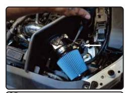
**25.** Install the air filter to the intake tube and secure using 8mm nut driver.
