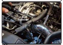
**23.** Once positioned and adjusted properly, secure the intake tube to the urethane hose. Tighten all clamps using 8mm nut driver.
