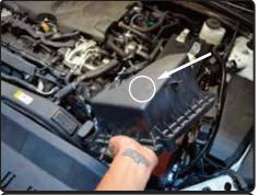
**6.** Un-clip the upper half of the air box and remove the stock intake assembly out of the vehicle.
