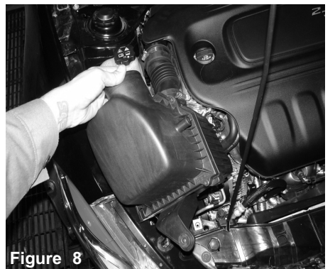
Figure 5 Pull back the crank case line from the air box.
