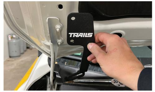
2. Working one side of the hood at a time, apply pressure to hood bracket while removing the (2) 12mm nuts. Place bracket on as shown, and thread 12mm nuts on by hand.
