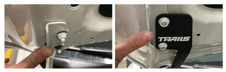
3. Tighten both 12mm nuts and check clearances before closing hood.
