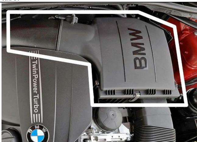
4. Carefully pull up and remove the upper and lower air cleaner assembly from the engine bay.
