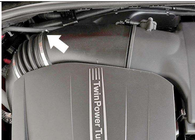
2. Loosen the hose clamp on the air intercooler pipe tube.
