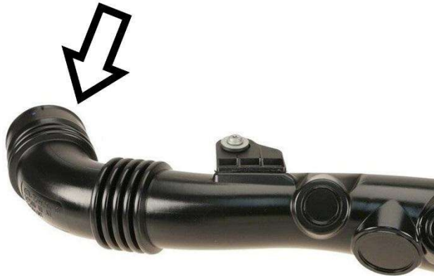
8. Loosen the hose clamp at the front of the charge pipe. The factory charge pipe can now be removed from the vehicle.
