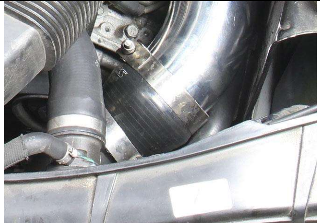
11. Install the silicone reducer onto the intercooler outlet pipe and secure it using the T-bolt clamp provided.
