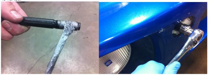
3. Depending on the model, you may need to use one or two spacers that are included in the kit to properly space the U-bracket from the bumper cover. Using the M6x25 bolt, thread it into the tow hook bolt with the U bracket and spacers (as needed) in between. The spacers (as needed) will be placed between the tow hook bolt and the U bracket. Loosely tighten with a 5mm hex wrench.
