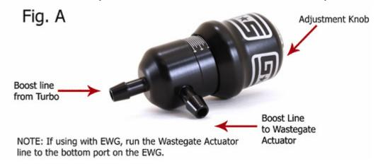
10. Turn adjustment knob CLOCKWISE to INCREASE boost pressure. Turn adjustment knob COUNTER-CLOCKWISE to DECREASE boost pressure (see end of adjuster for correct rotation direction). We advise starting at a lower boost pressure and then working your way up to your desired target boost pressure. Each click equals approximately one quarter of a psi. Each rotation equals one line on the scale and there are 16 clicks per rotation.
