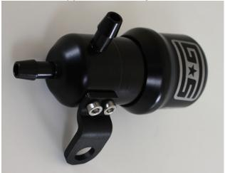
2. Find a proper location in the engine bay to mount the manual boost controller. You can either use the included bolt and nut (for through hole mounting), reuse a factory bolt, or use a zip tie to attach the boost controller. Be sure to mount it away from anything that would rub against it and make sure it is not mounted too close to an exhaust manifold or other hot pipe.
