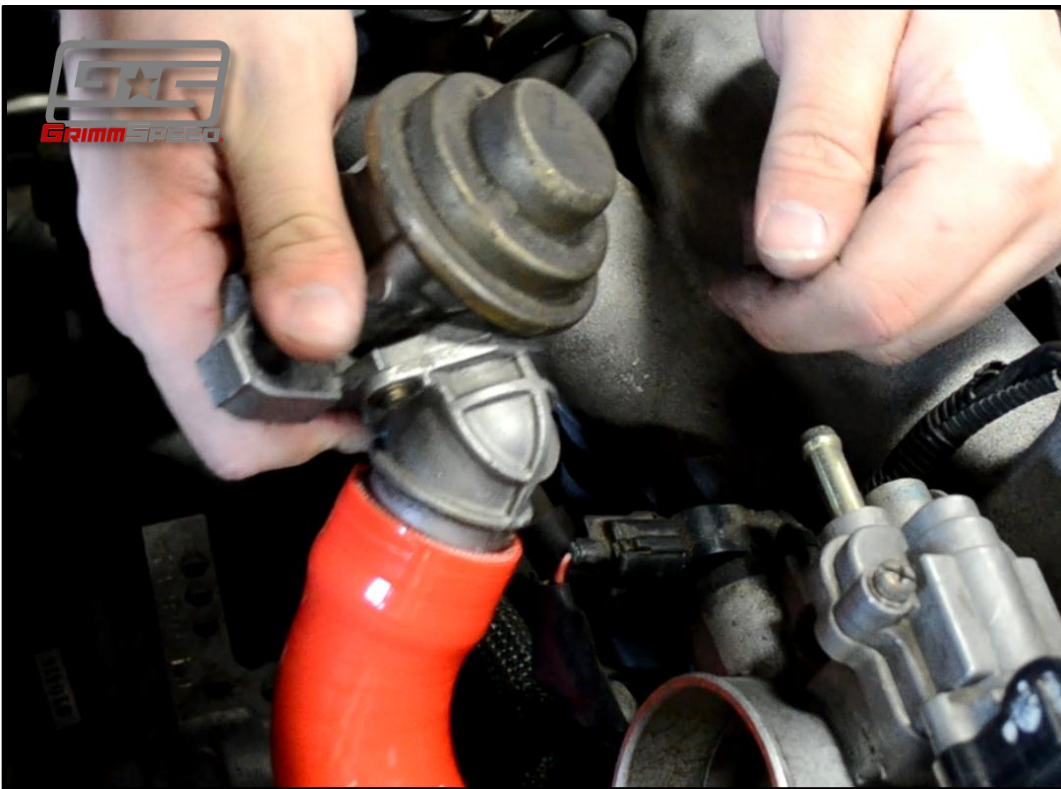
Figure 18: Install GrimmSpeed BPV hose
